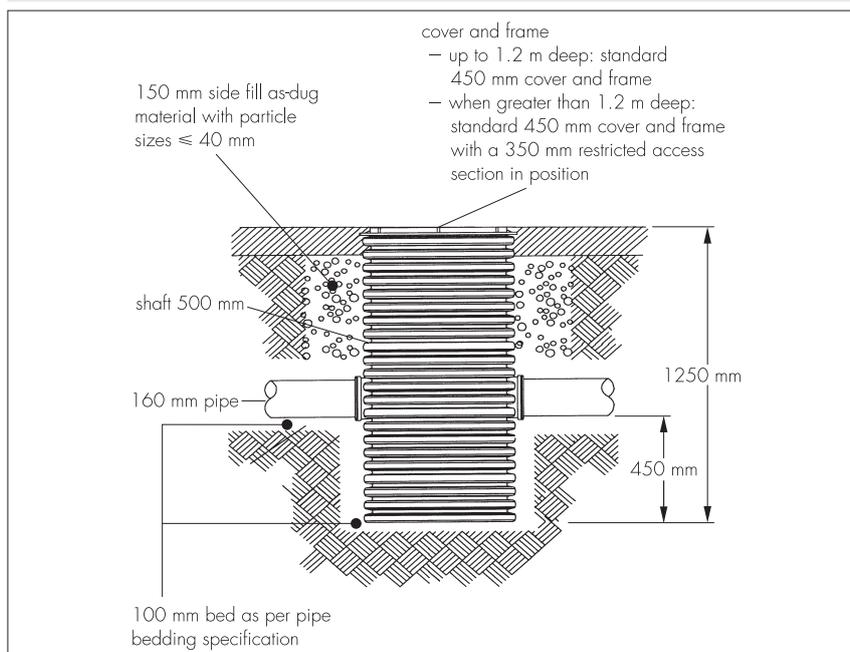
11.5 For all flow control devices it is sensible to incorporate access (via a manhole or similar) to the location of the pipe entry, orifice or vortex control. This will enable easy removal of any blockage. The orifice itself may be protected by a debris screen.
