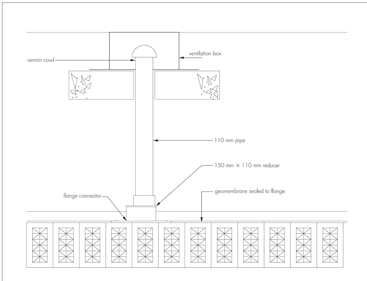
9.2 Typical air vent connectors and pipework can be seen in the Certificate holder's *Stormwater Solutions – Design Manual*. It is recommended that all air vent installations in attenuation/storage applications (using an impermeable geomembrane) are made using a flange adaptor. Adhesive or double-sided tape should be used between the geomembrane and flange adaptor to ensure a watertight seal.
